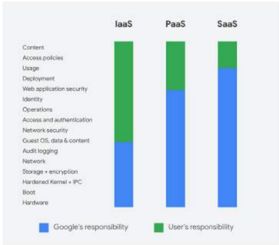
Google Workspace for Education (SaaS) responsibility diagram vs. other IaaS and PaaS services
